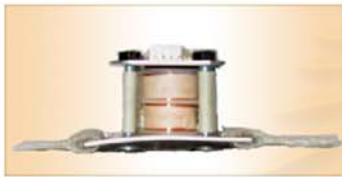
A vibrotactile actuator capable of producing up to 50 Hz signal
