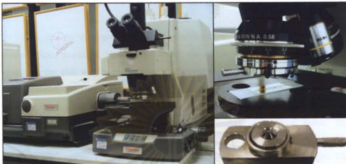
Figure 3.3 ATR FT-IR microscope: (A) Continuum ® infrared microscope coupled with the Nicolet 6700 FT-IR spectrometer, (B) the slide-on Ge \mu IRE is fixed on the position of slide-on housing on the infrared objective, and (C) Homemade slide-on germanium (Ge) \mu IRE.
