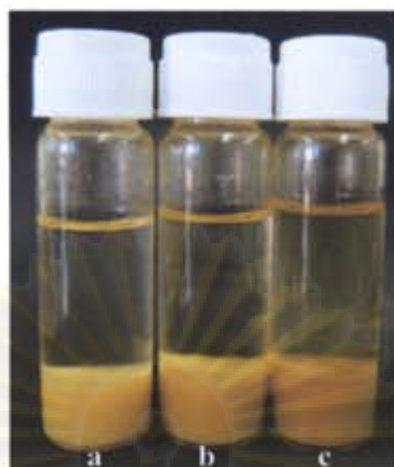
Figure 4.13 The deposited silver nanoparticles on silk sericin microparticles with concentrations: (a) 50, (b) 100, and (c) 200 ppm.
