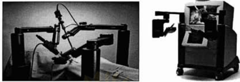
Figure 2.2: Three arms at a patient-side and a surgeon console of The ZEUS™ Robotic Surgical System [4]
