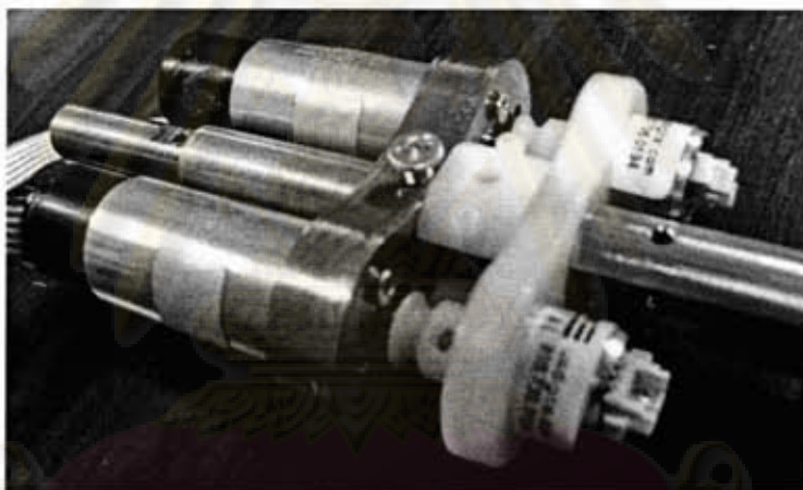
Figure 3.21: The 5 th and 6 th actuators with absolute encoders
