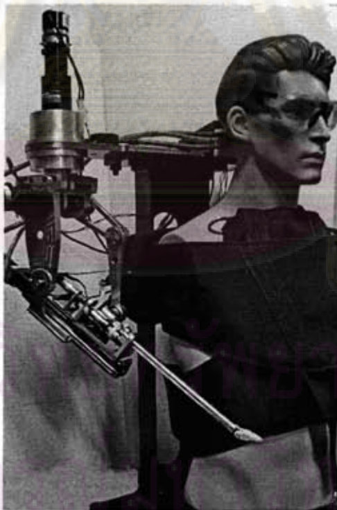
Figure 3.24: The RCRT-1 Manipulator with the human figure
