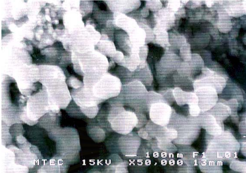
Figure 4.6 SEM micrograph of SnO 2 raw material. The average particle size of SnO 2 raw material is in the range of 50-200 nm and the shape of SnO 2 powder is spherical.
