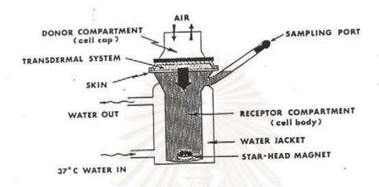
Fig. 10: Schematic of Modified Franz Diffusion Cell.
