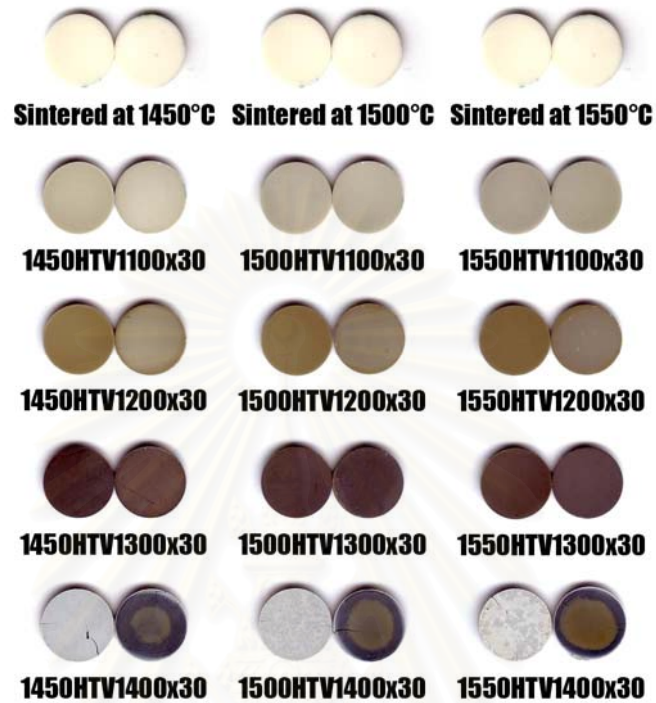
Figure 4.6 Colors of specimen sintered at 1450-1550°C and annealed at 1100-1400°C with a soaking time of 30 min, top side (left) and bottom side (right)
