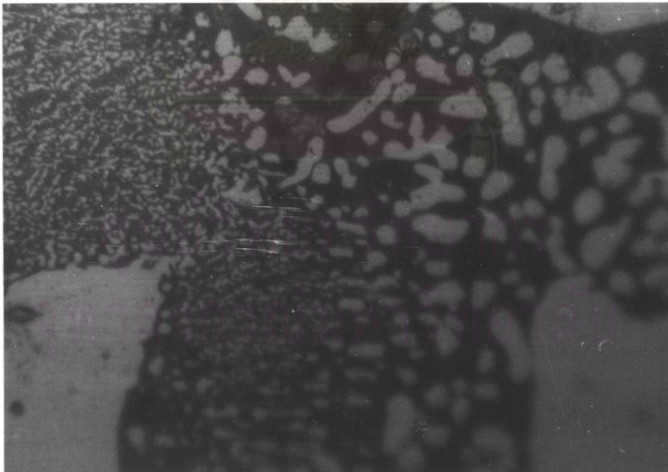
Figure B6 Ternary eutectic structure of \text{FeO-Fe}_2\text{SiO}_4\text{-Fe}_2\text{O}_3 and dendritic structure in H-32 sample, x500.
