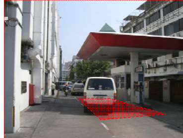
Location of Underground Diesel Tank on the 1 st FL. at the back of BBL building for New Generator. (@ 28,000litres x 2)
