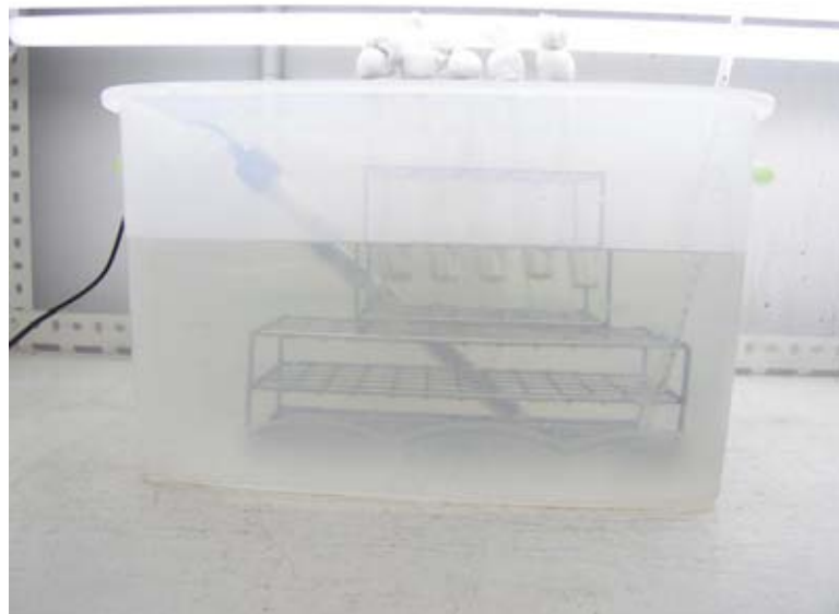
Figure 3-6. Temperature control unit for W. globosa grown in various temperatures for photosynthesis study
