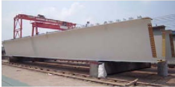
Figure 4.3 Steel box girder
