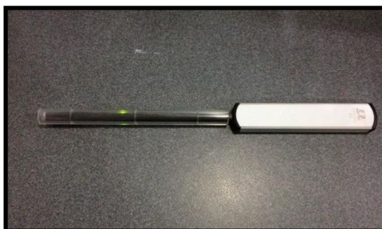
Figure 3.4 The pencil-type ionization Unfors RaySafe Xi CT Detector
