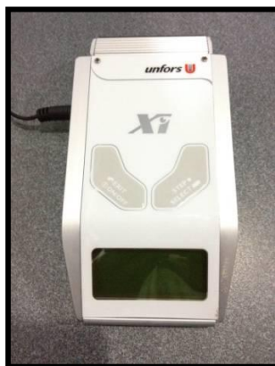
Figure 3.3 Unfors RaySafe model Xi platinum dosimeter
