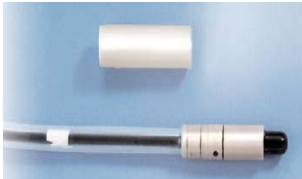
Figure 3.4. 0.13 \text{ cm}^3 cylindrical ionization chamber type CC13.
