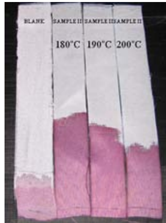
Figure 4.7 Wetness of untreated polyester fabric and treated polyester with phthaloyl chitosan (chitosan ( M_w=10^6 ):PA =1:18; concentration 9 g/l)
