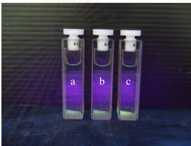
Figure 3.7 Photograph of the ion exchange support after treatment with a) PNA alone (control) b) PNA + single mismatched DNA c) PNA + complementary DNA.
