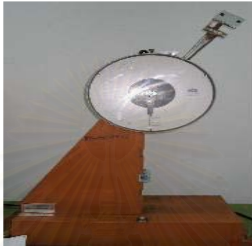
Figure 3.4 ATS Charpy Impact Tester
