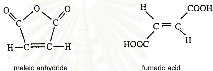
Figure 2.5 Chemical structures of maleic anhydride and fumaric acid
