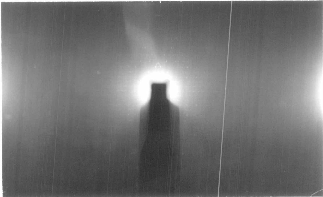
Fig. 3.4.2 Oscillation photograph of \text{Nb}_3\text{As} rotated about a axis \text{MoK}_\alpha radiation, for 12 hours exposure.
