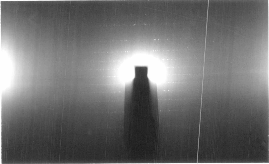
Fig. 3.4.1 Oscillation photograph of \text{Nb}_3\text{As} rotated about c axis \text{MoK}_\alpha radiation, for 12 hours exposure.
