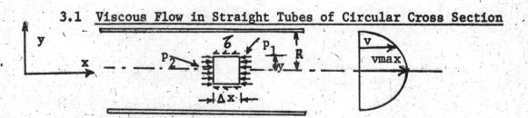
Consider the cylindrical fluid element of length dx and radius y as shown above.
