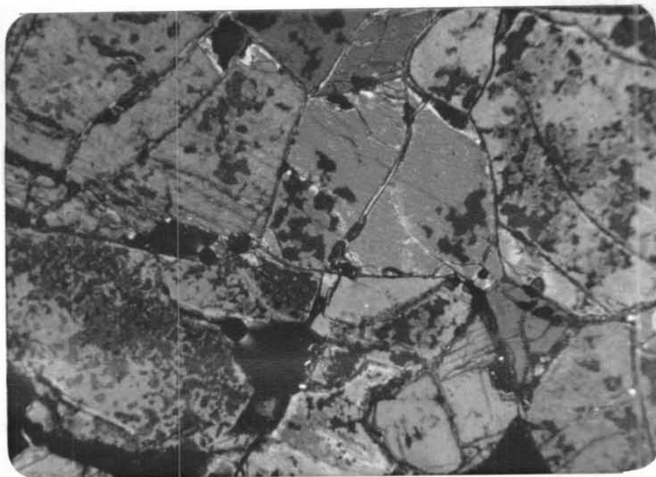
Figure 16 Photomicrograph of spinel-lherzolite inclusion, (cross-nicols, magnification 40 x)
