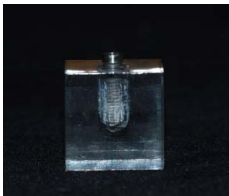
Figure 12 The implant body was embedded in the acrylic block.
