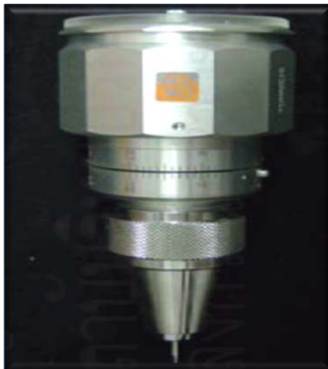
Figure 20 The screw driver was fixed in the three jaw chuck of the torque gauge.
