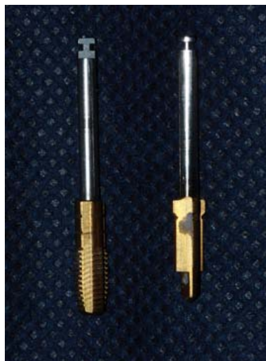
Figure 10 The instrument of CU dental implant for acrylic block preparation
