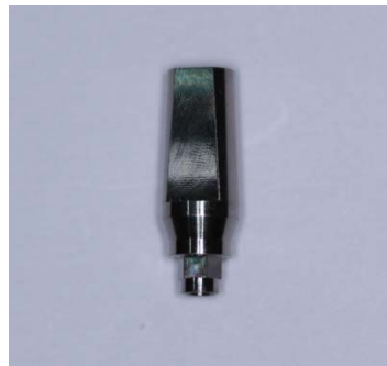
Figure 15 The abutment from CU dental implant
