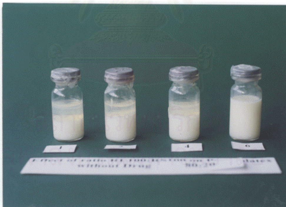
Figure 17 Effect of ratio RL100 : RS100 = 80 : 20 on water removal time of pseudolatex without drug at 1, 2, 4, and 6 hours, respectively (settle for one month).
