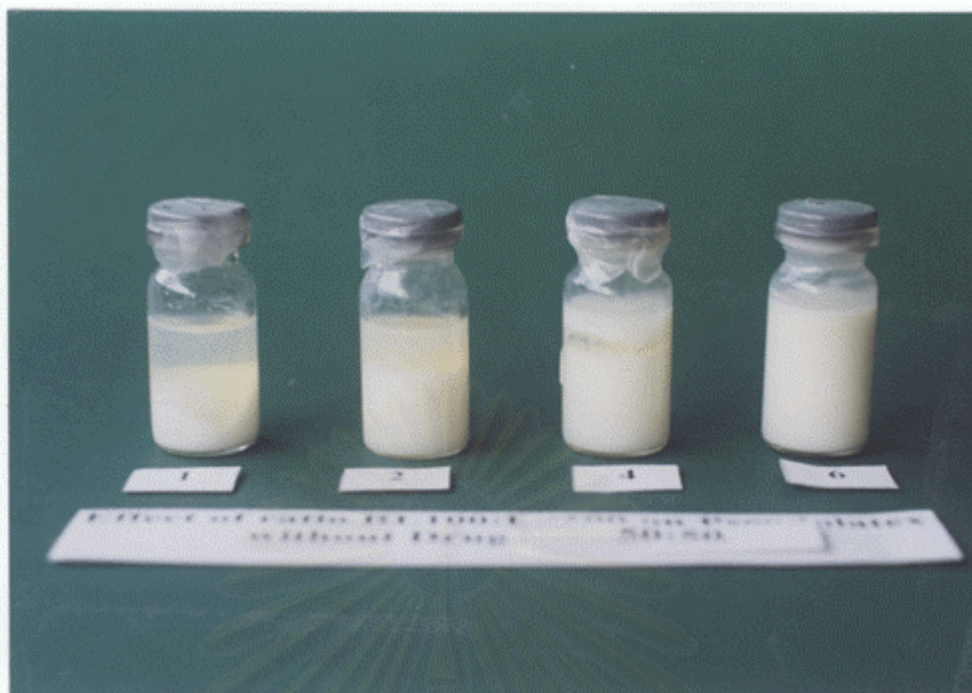
Figure 18 Effect of ratio RL100 : RS100 = 50 : 50 on water removal time of pseudolatex without drug at 1, 2, 4, and 6 hours, respectively (settle for one month).
