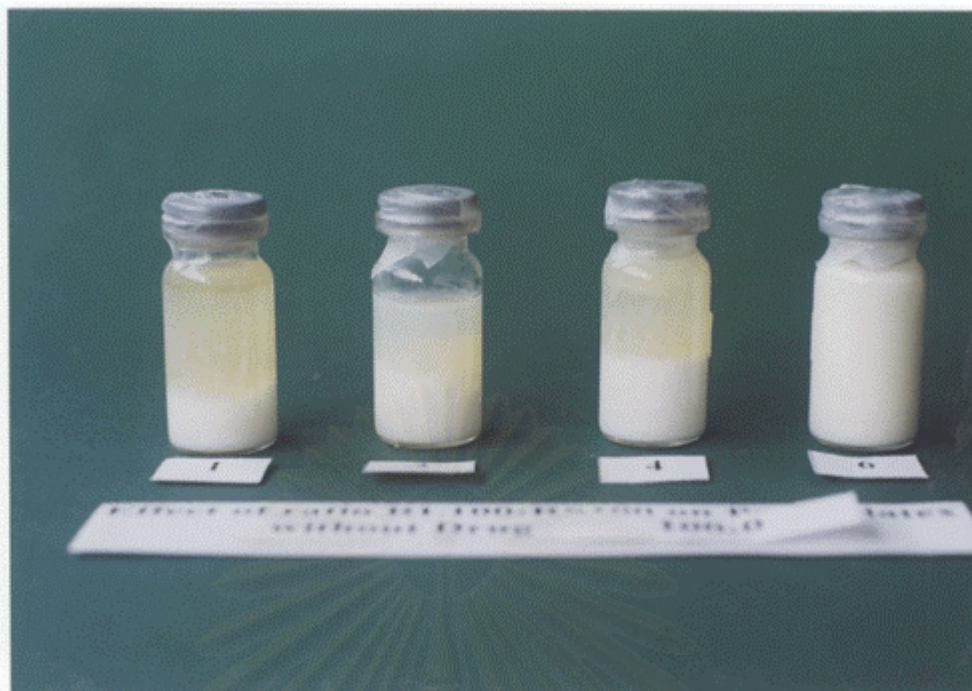
Figure 16 Effect of ratio RL100 : RS100 = 100 : 0 on water removal time of pseudolatex without drug at 1, 2, 4, and 6 hours, respectively (settle for one month).
