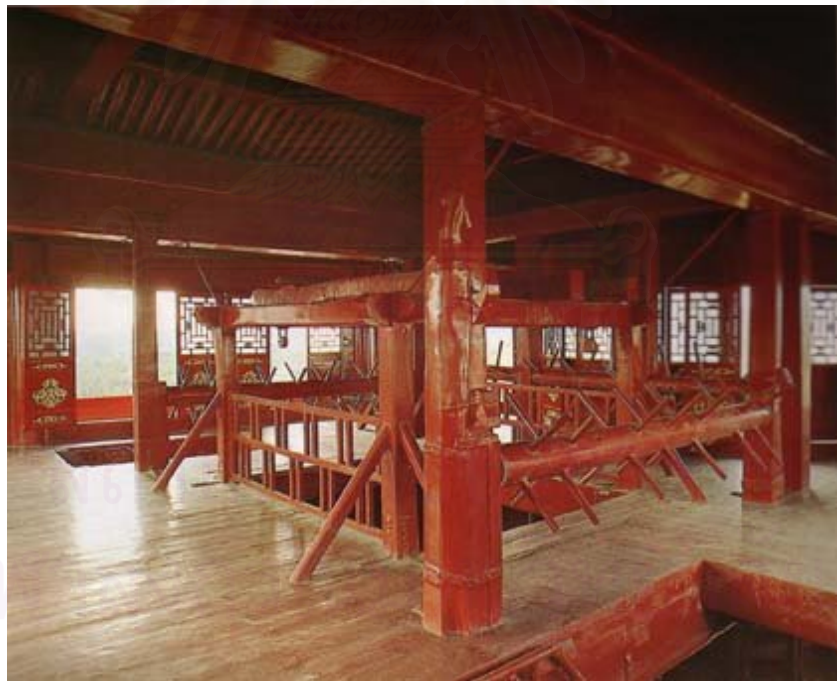
Pic. 14. Five handspike windlasses for the lifting apparatus located in the backstage of the Fortune Stage of the Pleasant Sound Pavilion. Photo from Yu Zhuoyun, Zijin Cheng Gongdian , p. 166, plate 184.
