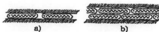
Figure 2.1 Alkyl chain aggregation in layered silicates: a) lateral monolayer; b) lateral bilayer (Vaia et al. , 1994).
