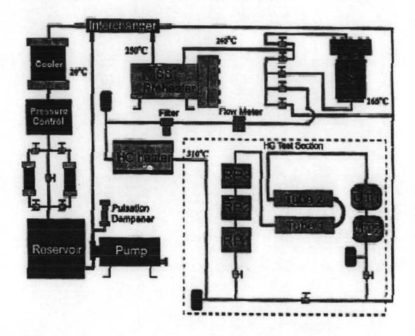
**Figure 3.1** The schematic diagram of simulated primary coolant system of CANDU reactor (Cook, 2000).
