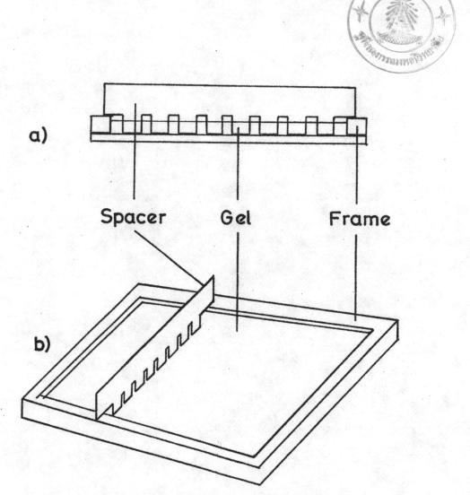
Figure 3. Gel tray and spacer,
