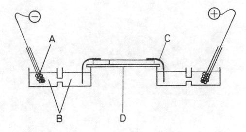
Figure 2. General layout of the electrophoresis apparatus.
