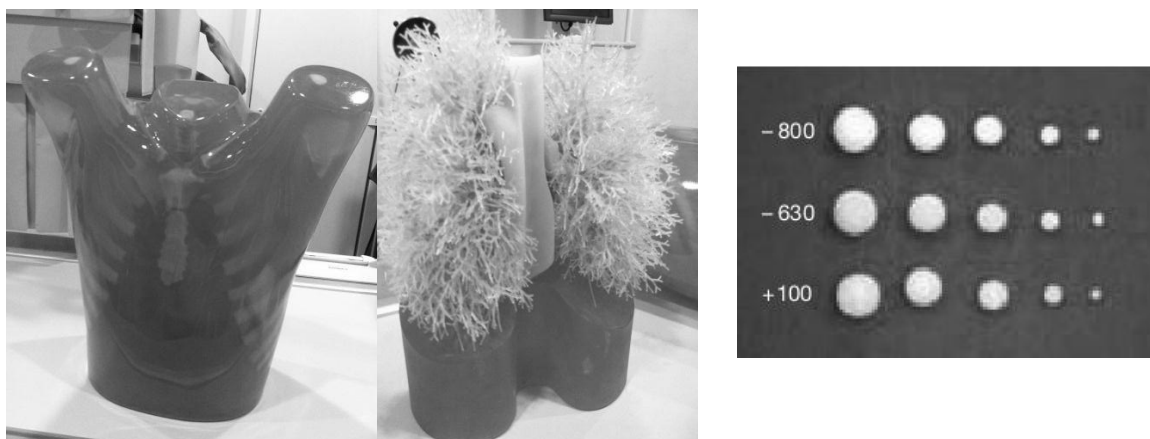
Figure 3.5 Multipurpose chest phantom N1 LUNGMAN and simulation circular nodules in five sizes and three HU units number.
