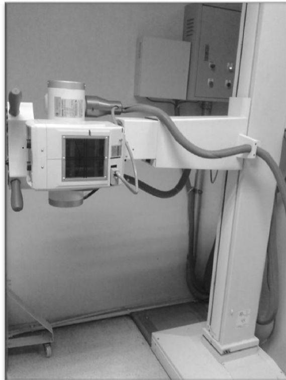
Figure 3.4 TOSHIBA x-ray tube housing model ROTANODE.
