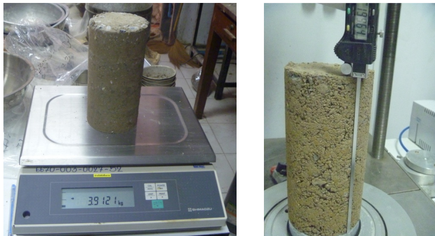
Figure 3.4 Weighting compacted sample (Left), compacted sample size measurement (Right)
