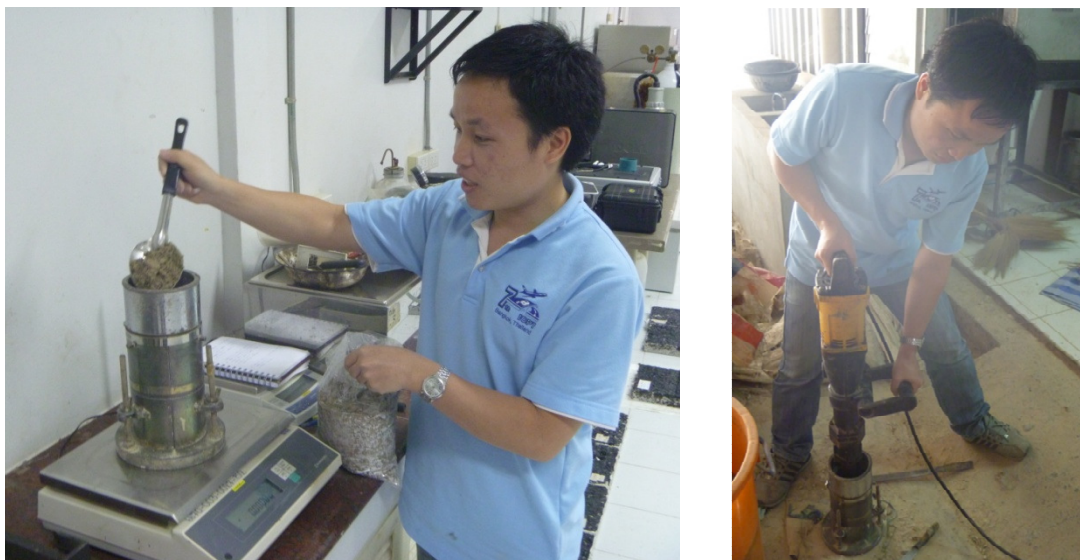
Figure 3.3 Weighting sample for one compact layer (Left), during compaction (Right)
