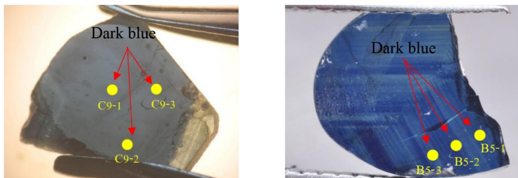
Figure. 5.6 Analytical spots on dark blue zones after heating at 1650 °C in samples C9 (left) and sample B5 (right).
