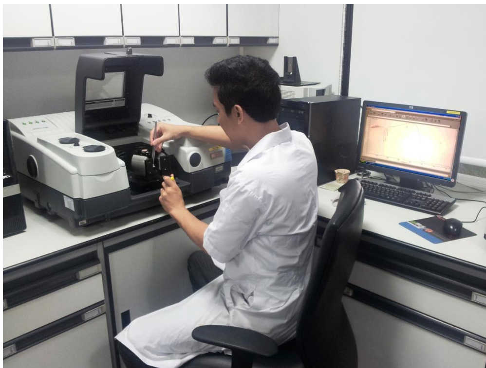
Figure 1.6 Thermo Scientific Fourier Transform Infrared (FTIR) Spectrometer (Model Nicolet 6700) at the GIT
