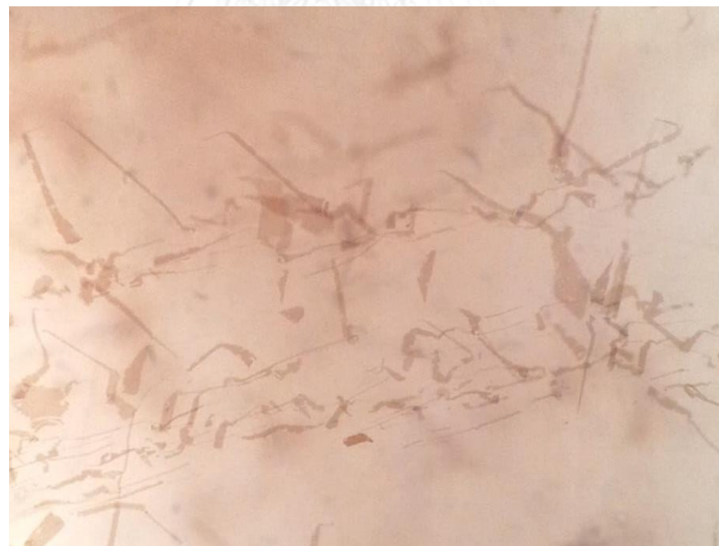
Figure 3.8 Photomicrograph with high magnification (using combination of reflected and transmitted lights) showing irregular lamellae feature of silky inclusions orientated along crystallographic directions in sample C9; indication of subsolidus exsolution of the sapphire host.
