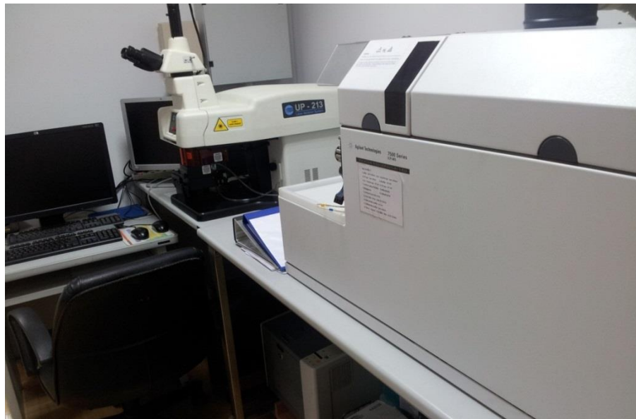
Figure 1.8 Laser Ablation-Inductively Coupled Plasma-Mass Spectrometry (LA-ICP-MS) based at The Gem and Jewelry Institute of Thailand.
