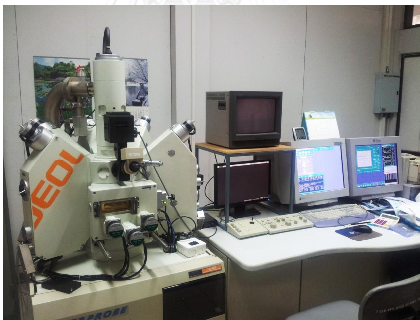
Figure 1.4 JEOL Electron Probe Micro-Analyzer (EPMA) model JXA 8100 based at Department of Geology, Chulalongkorn University
