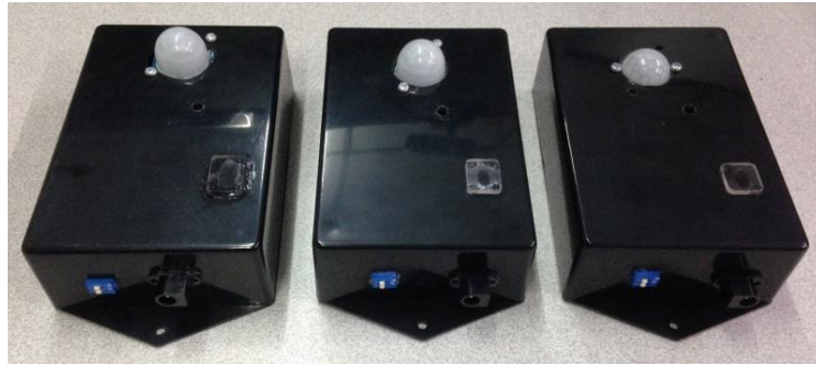
Figure 60 6LoWPAN Client Nodes using in system
