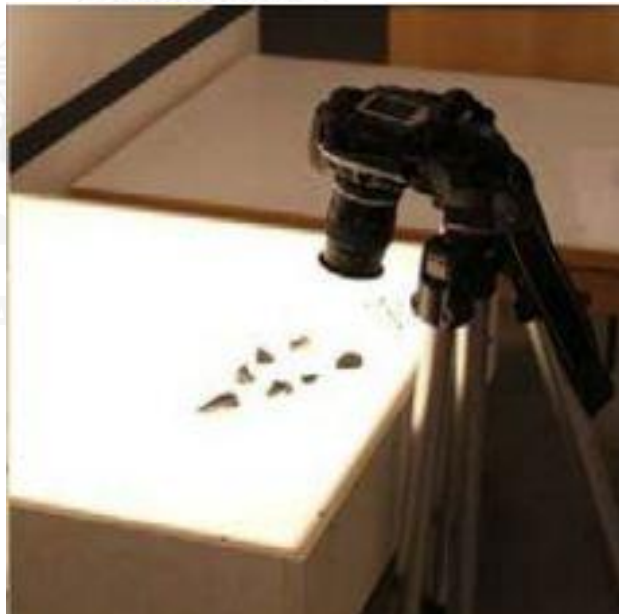
Figure 2.6.4 An SLR camera was used to take the images of the soil sample (Rodriguez et al., 2012)
