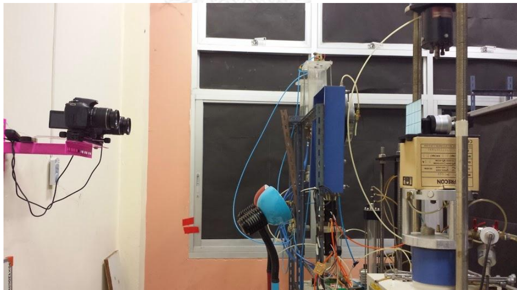
Figure 3.3.5 Experimental set up for determining the accuracy with respect to the triaxial apparatus
