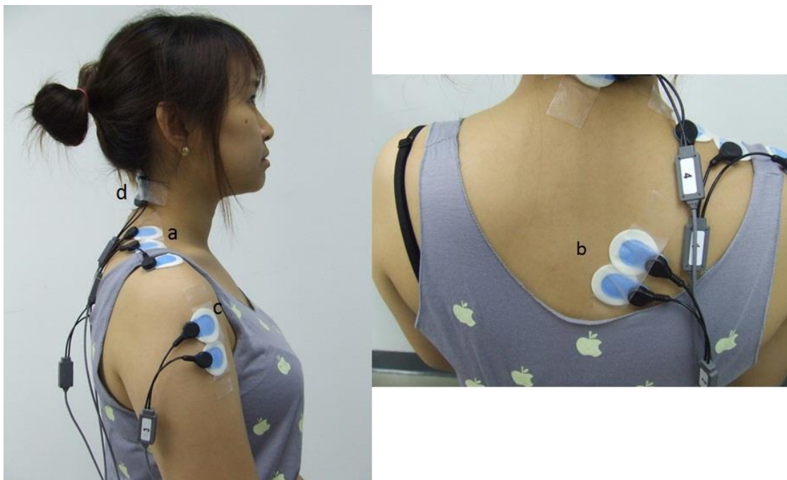
Figure 5.1 Electrode placement: a) Upper trapezius; b) Lower trapezius; c) Anterior deltoid; d) Cervical erector spinae
