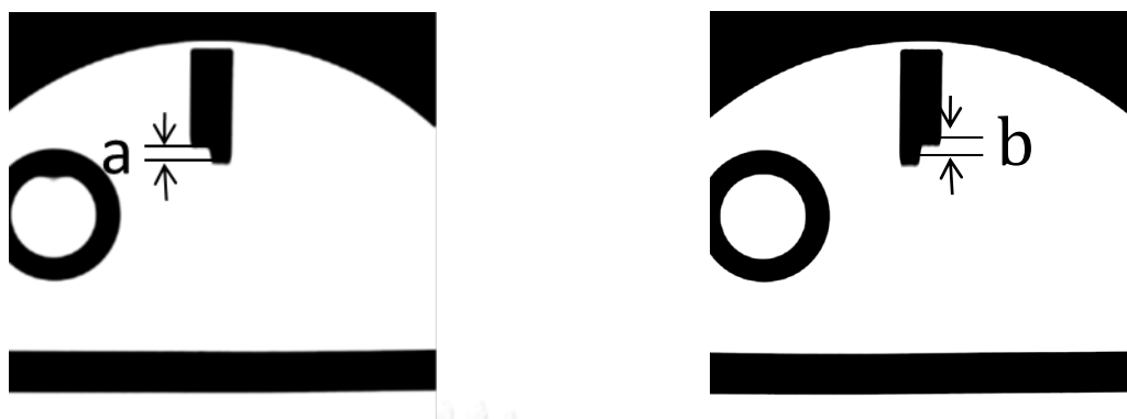
Figure 7.5 Images of slice 1 illustrating measurement of slice position error. The arrows indicate the bar length difference measurement that is to be made.
