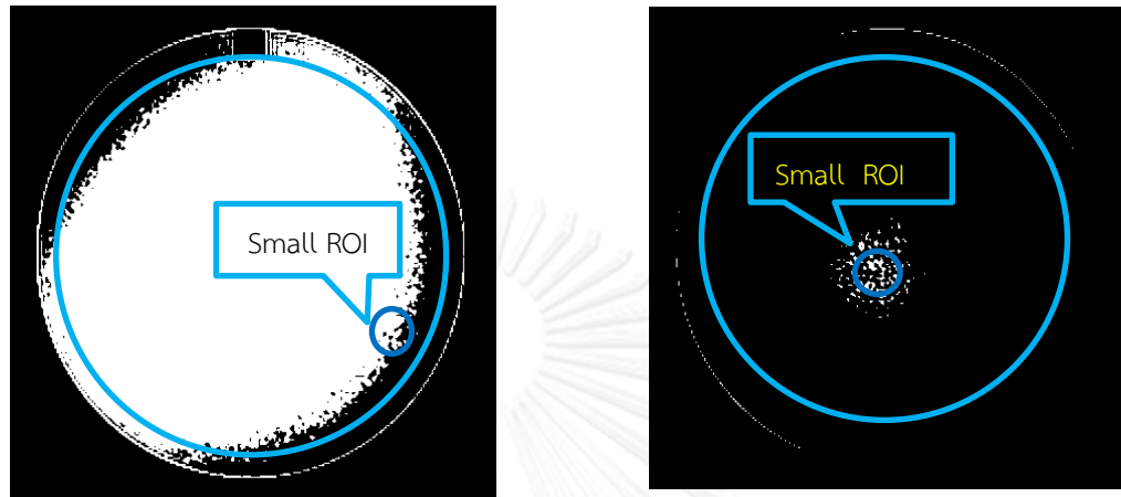
Figure 7.6 (right) ROI placement for low signal-value, (left) ROI placement for HIGH signal-value.
