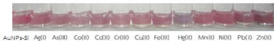
Figure 4.14 The solid phase color after extraction and detection of Hg(II) (0.025 $\mu$ M) and various metal ions (2.5  $\mu$ M).
