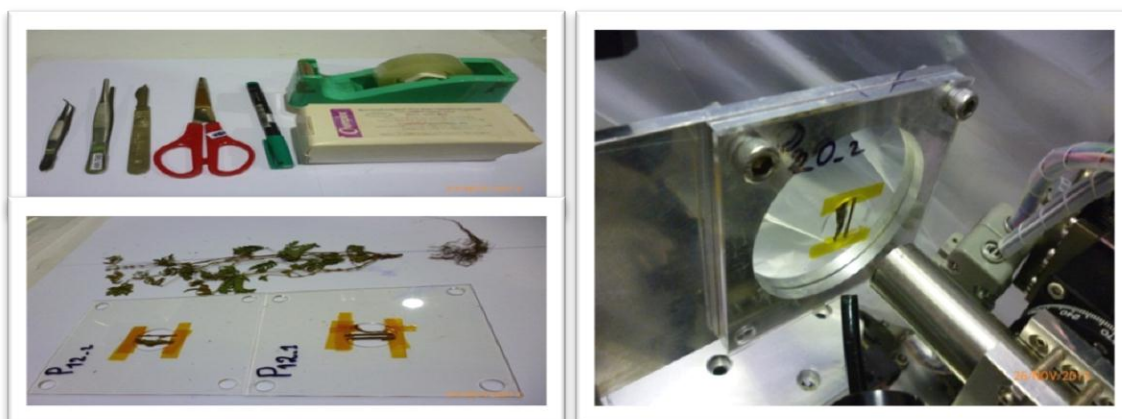
Figure C-8 Sample preparation and analysis by the microbeam synchrotron X-ray fluorescence beamline
