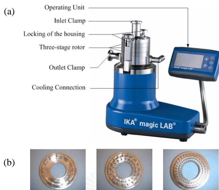
Fig.4.4 (a) HSM (Magic-Lab, IKA) and (b) Three types of rotor; coarse, medium and fine rotor, respectively.
