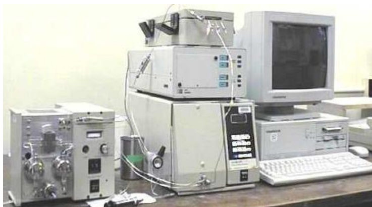
Figure 3.5 High performance liquid chromatography (HPLC).
