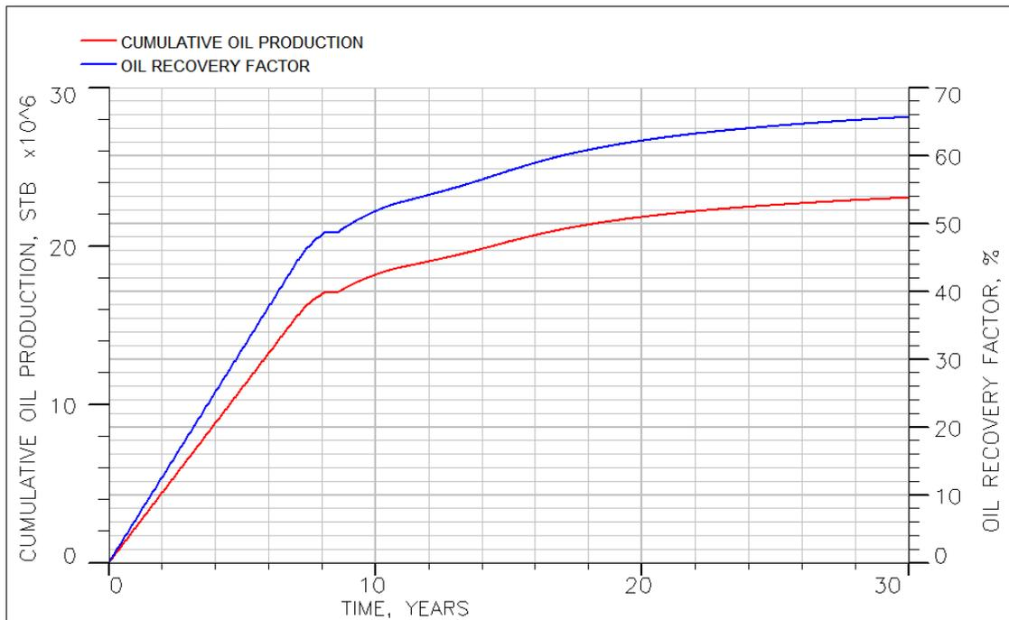
Figure 5.15 Cumulative oil production and oil recovery factor of the WAG with down-dip injection base case.
