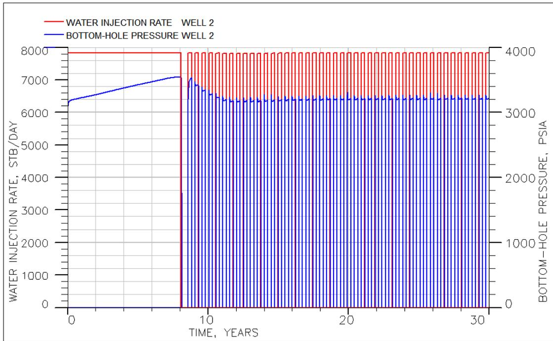
Figure 5.12 Water injection rate and bottom-hole pressure of water injector of the WAG with down-dip injection base case.
