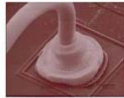
1 st bond of Good IC (pin#13)
