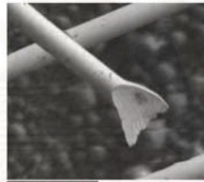
Wire tail of cracking
