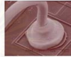
1 st bond of Good IC (pin#12)
