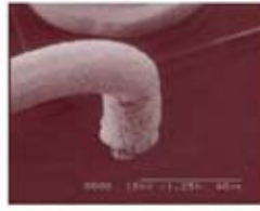
The wire neck of defect
