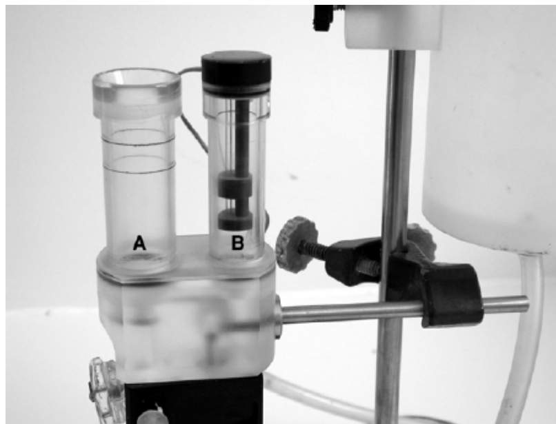
Figure 9 Plethysmometer. The larger one (A) is used to measure fluid displaced by the paw, a volume change that is precisely mirrored in the smaller tube (B) containing a transducer which is linked to a decoder capable of digitally displaying volumes.
