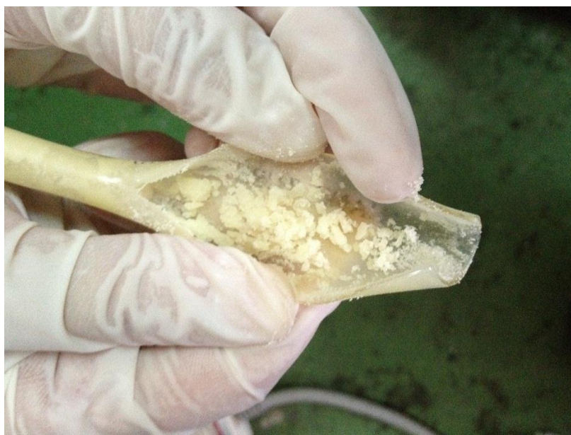
Figure A.2 Clogged soap stuck in the silicone tube after product was drained.
