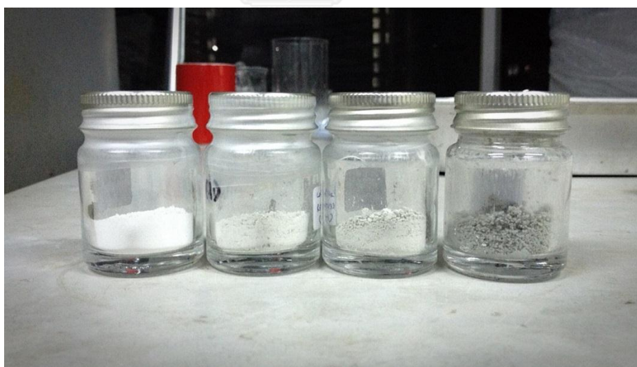
Figure A.4 The fresh, 1 st cycle, 2 nd cycle and 3 rd cycle of calcium oxide catalyst (from left to right, respectively) after washed and dried to remove methanol.
