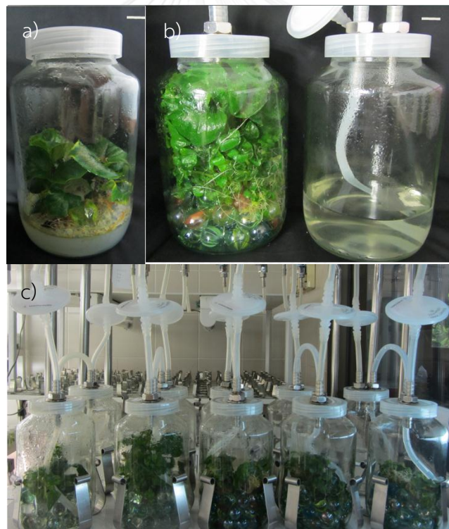
Figure 21 Comparison between conventional method (CM) and temporary immersion bioreactor (TIB) of Ophiorrhiza harrisiana tissue cultures.
