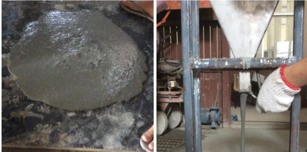
Figure 3.3 Slump flow test details
