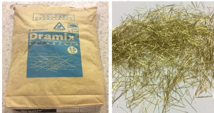
Figure 3.2 Steel fibers used in UHPFRC slabs
