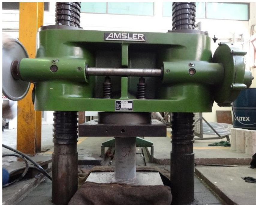
Figure 3.5 - Cylinder compressive test set up
