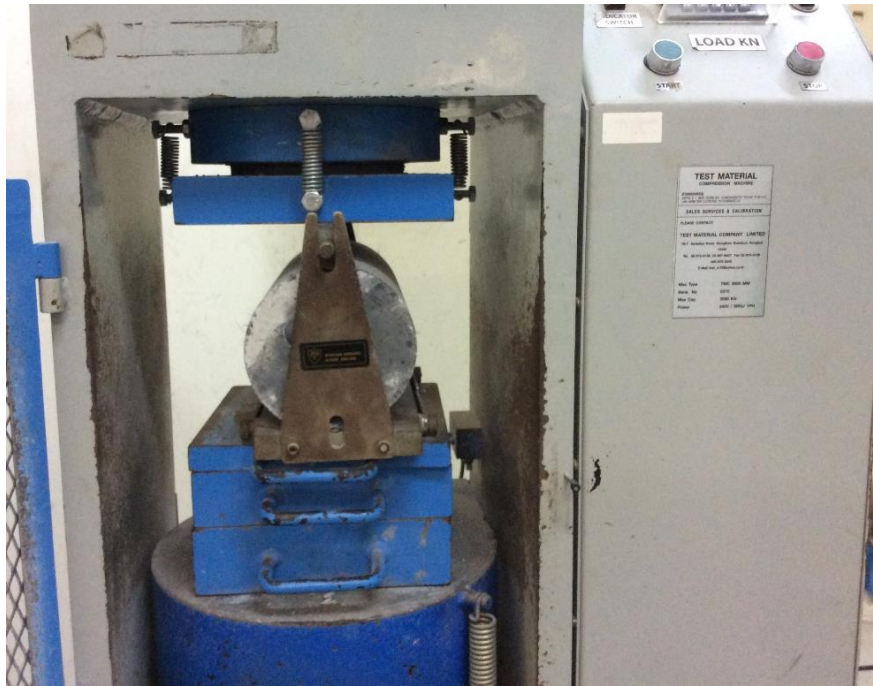
Figure 3.6 Cylinders splitting tensile test set up
