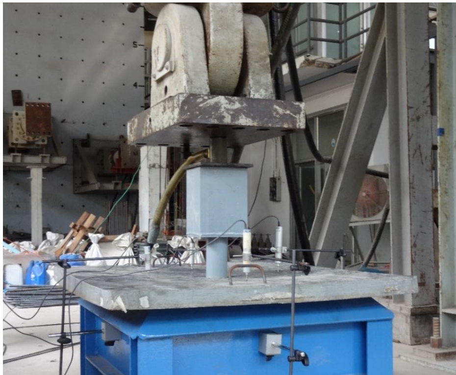
Figure 3.14 Punching shear test setup of UHPFRC slabs
