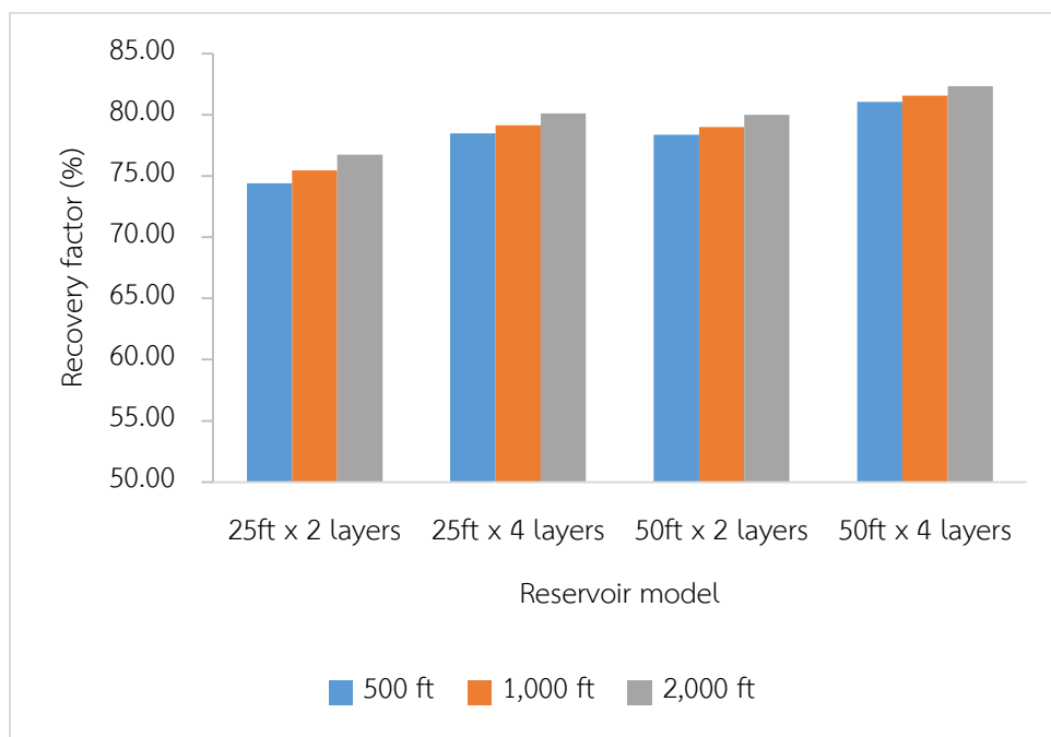
Figure 5.46 Recovery factor of each reservoir model and various depth differences between oil and topmost gas reservoirs
