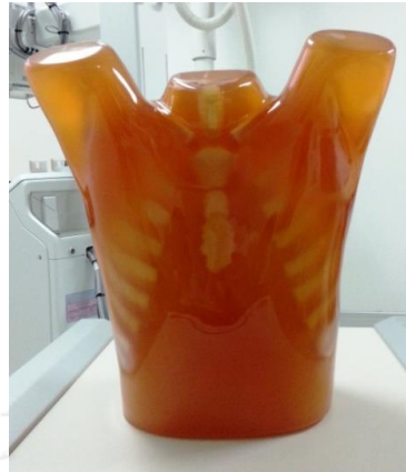
Figure 3.4 Multipurpose chest phantom N1 LUNGMAN.
