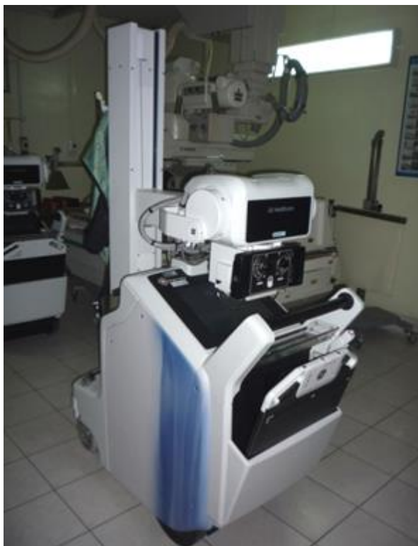
Figure 3.1 Digital mobile x-ray GE Optima XR220amx and Digital image receptor.
