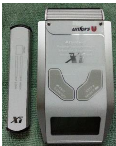
Figure 3.3 Solid state dosimeter manufacturer UNFORS RaySafe model Xi.
