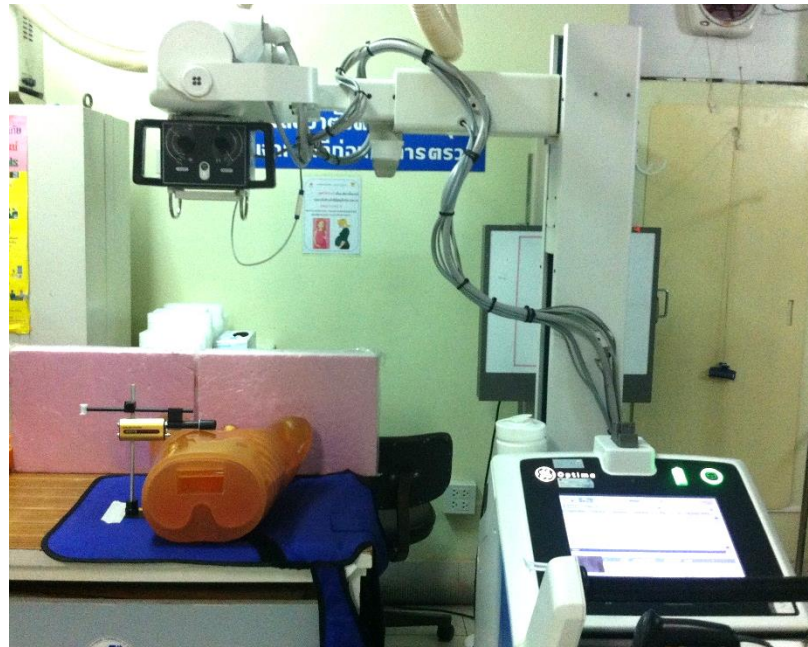
Figure 3.7 Set up for the entrance surface air kerma, K_e measurement
