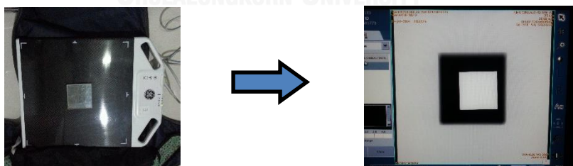
Figure 5: Lead glass and image after exposure
