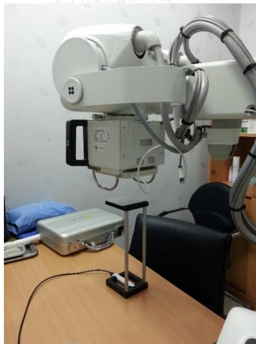
Figure 3.5 Set-up for quality control of x-ray beam quality.
