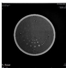
Figure 11: Obtained image form TO20 test tool.
