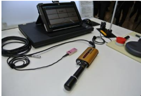
Figure 3.2 Ionization Chamber dosimeter manufacturer Radcal model AGDM.
