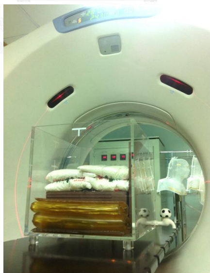
Figure 3.12 CT scanning of water equivalent phantom.
