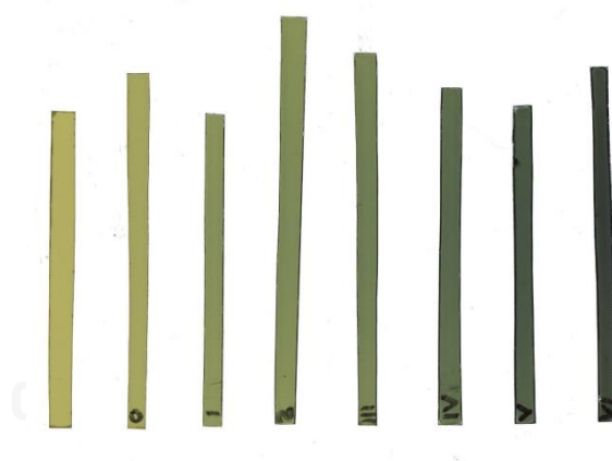
Figure 3.16 The 8 irradiated film strips with the different dwell time for different doses.
