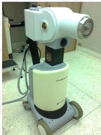
Figure 3.3 High dose rate Brachytherapy machine.
