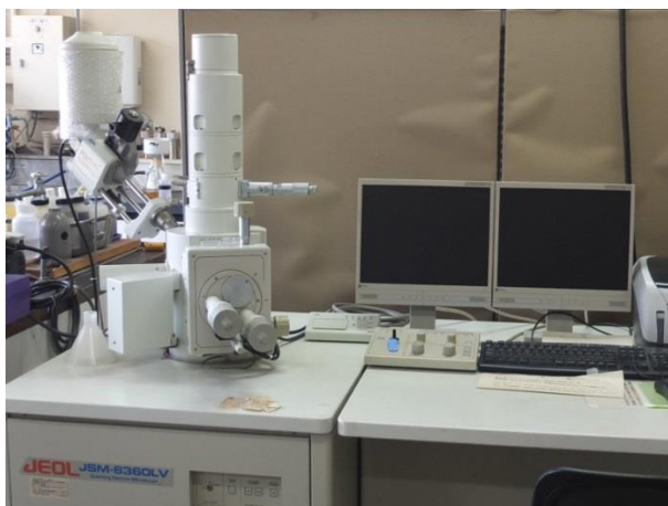
Figure 11 Scanning electron microscopy (SEM: JEOL, JSM-6360LV)
