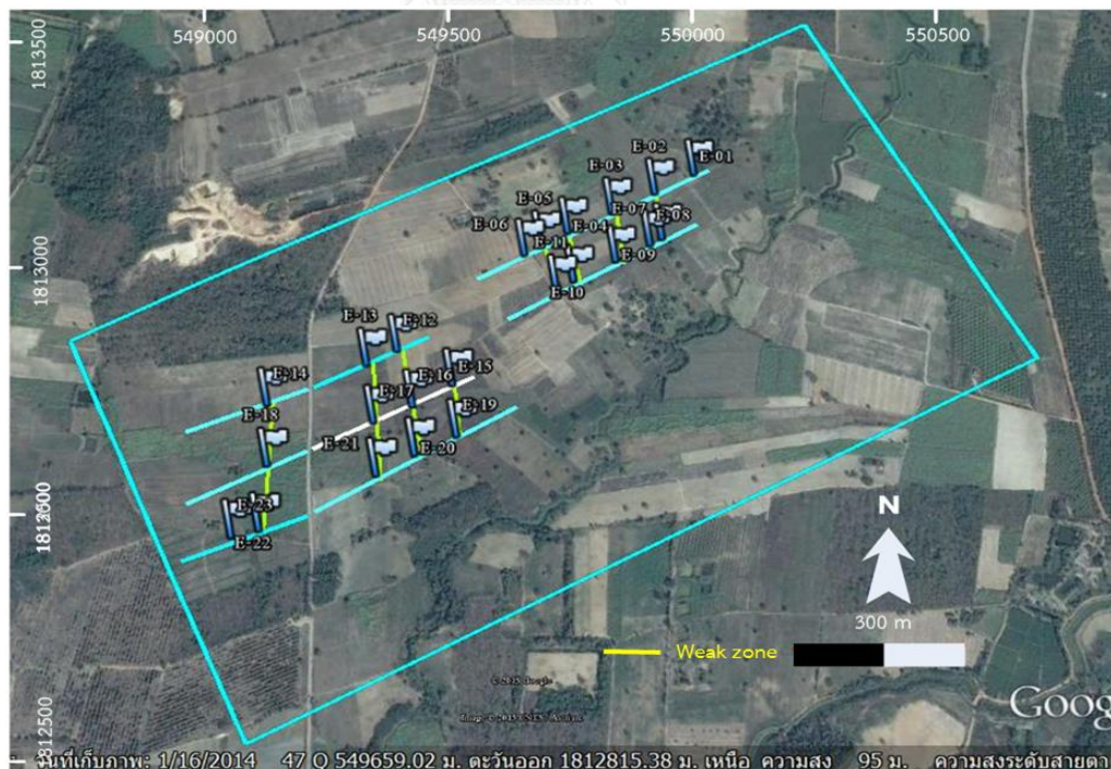
Figure 5.2-1. The potential groundwater expected location points and weak zones that are weathered phyllite or/and fracture zones in the study area.
