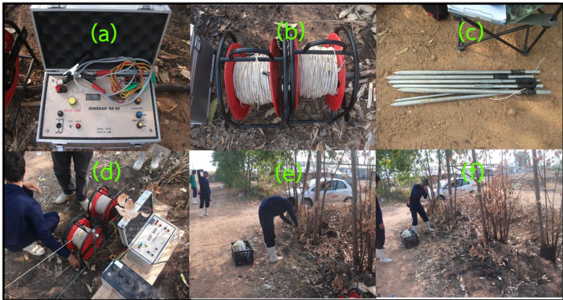
Figure 3.3-1. The VES instruments and survey method (a) control box measures voltage and current, (b) two cable rolls are connected with source electrode at cable terminal, (c) some electrode poles which have at least 1 pair is receiver electrode are connected with control box, and other pair is source electrode are connected with cable rolls, (d) instrument emplacement have battery, cable rolls, and etc., are connected with control box, (e) connecting cable and electrode pole and, (f) hammering the electrode pole to the ground.
