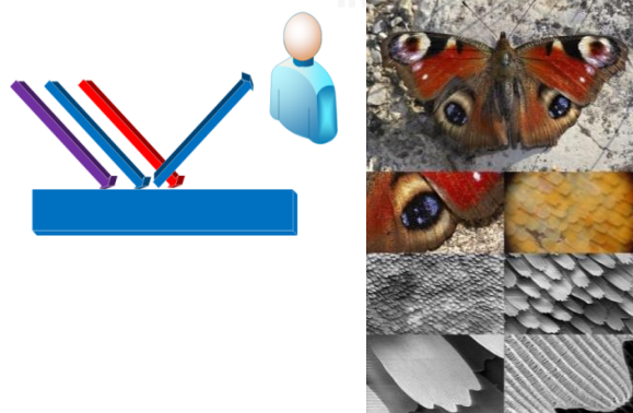
Figure 2.7 (Left) Observer detects blue spectrum from reflection of blue pigment (Right) Structural coloration on butterfly's wing
