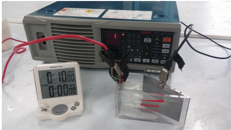
Figure 2.3 Classic trapezoidal Hull cell bath of electroplated zinc process in this project.
