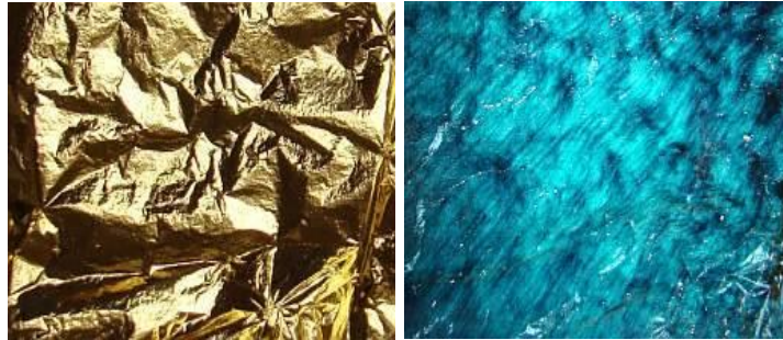
Figure 2.9 gold thin films (Left) gold color in normal ambient light (Right) gold color in light from behind the film.[13]
