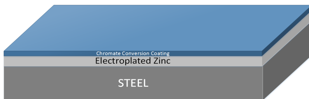
Figure 1.1 Schematic coating of electroplated zinc layer with CCC as top-coating on steel products
