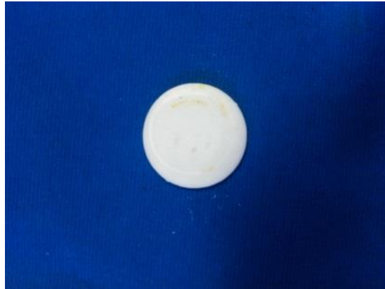
Figure 7 The specimen size 12 mm in diameter and 1 mm thick
