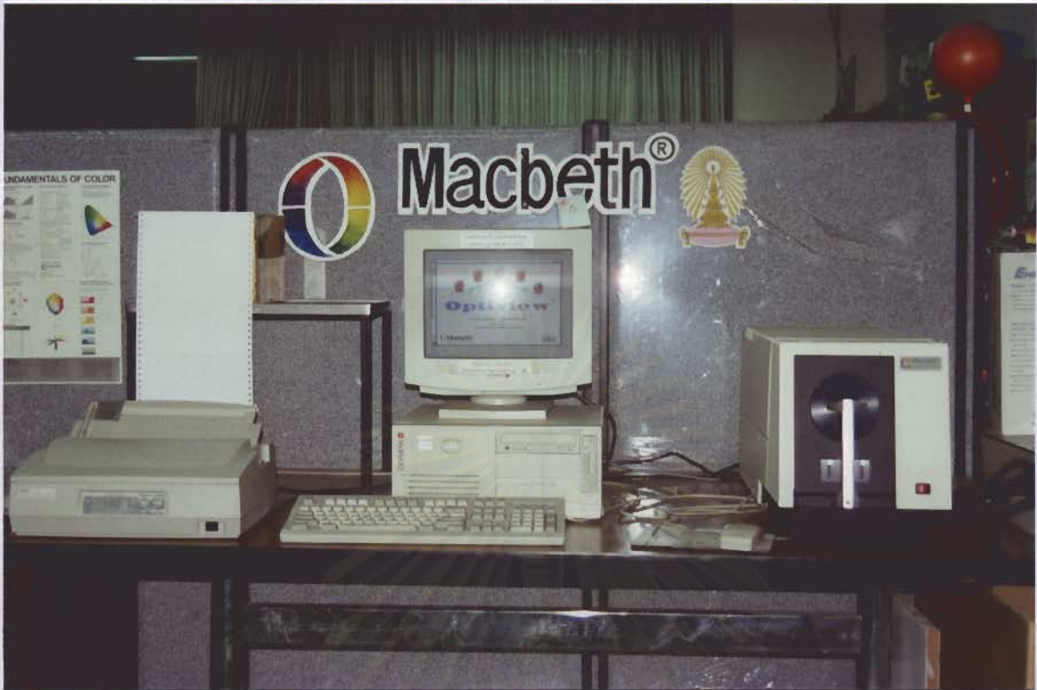
Figure A-3 Reflectance spectrophotometer: Gretag-Macbeth Color Eye 7000 and Optiview software.
