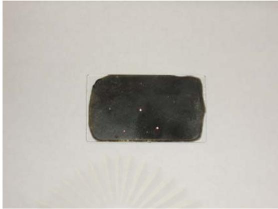
Figure A-10 Thin section samples for observation by optical microscope.
